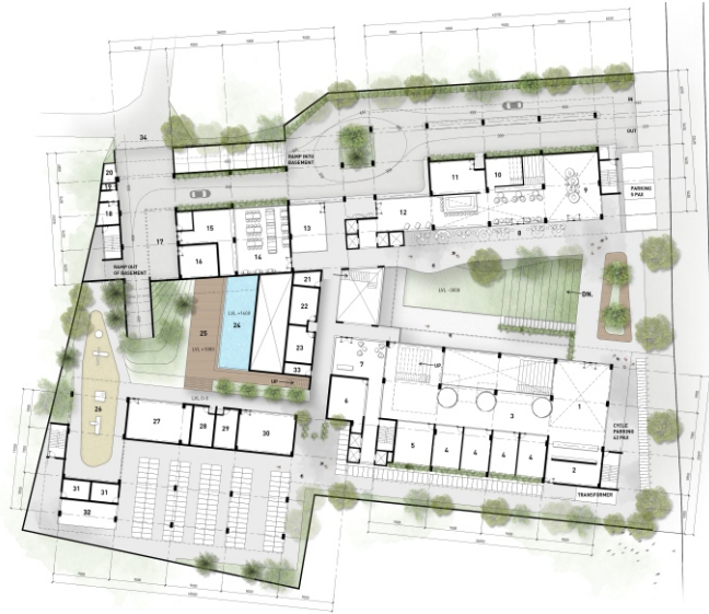
Ground floor plan - The central spine with pedestrian plaza, drop off to residences, bike parking, café and recreational spaces, children's play area, co-working space
