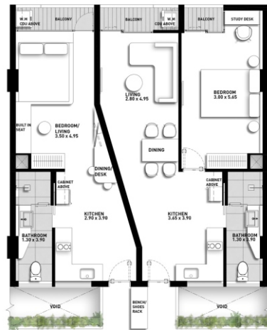
Studio and 1 bedroom cluster - The angled wall creates more space for the studio to accommodate the kitchen and dining, within the structural grid.
