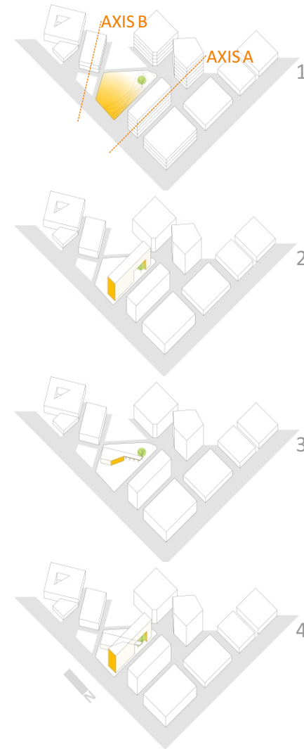
1-The site with a large tree. 2-Block A bridges over the tree while responding to the scale and alignment of the adjacent building. 3- Similarly, Block B responds to its adjacent building. 4- Block B connects with Block A by penetrating the atrium.
